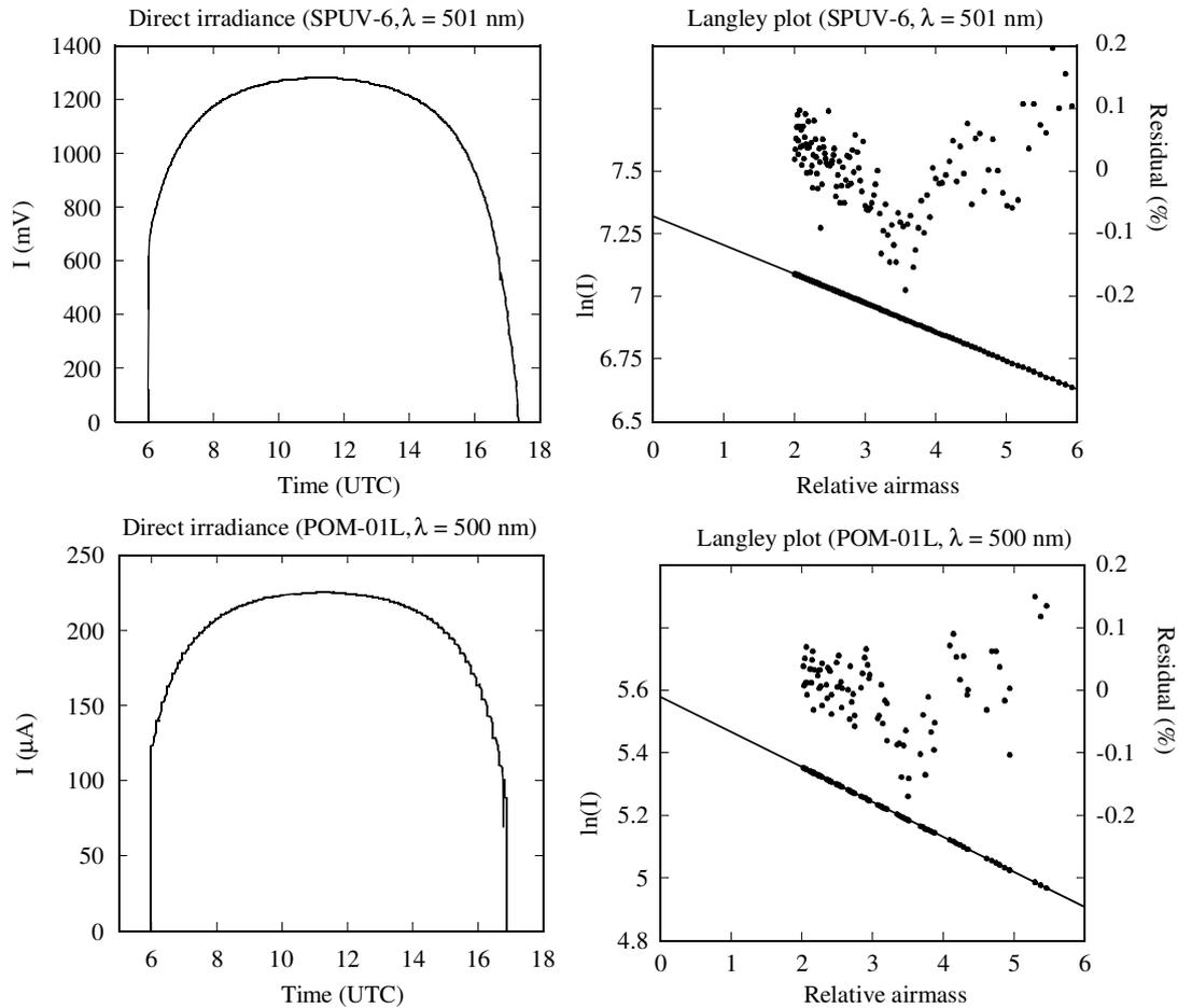
**Figure 2:** Direct irradiance measurements and Langley plots for the SPUV-6 (KNMI) and POM-01L (Kipp & Zonen) for 20 September 2003. The wavelength is 500 nm. The scattered points indicate the differences between the measurements and the fit, relative to the instrument signal.
